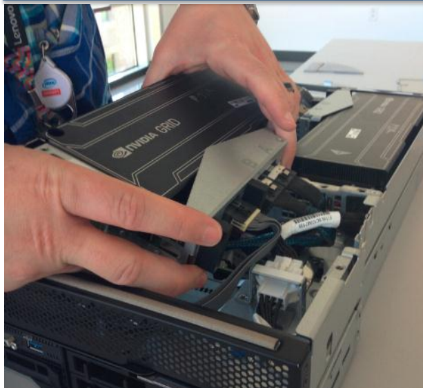
SD530 with cables ready for GPU node install
